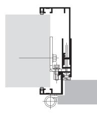
Aluminium frame type Hardline for dulled doors
